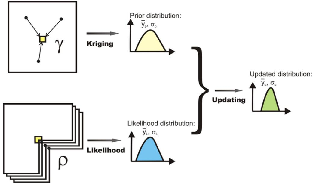
**Figure 1:** Schematic illustration of the Bayesian updating technique. The block dots are data, and the yellow square is a location being estimated.
