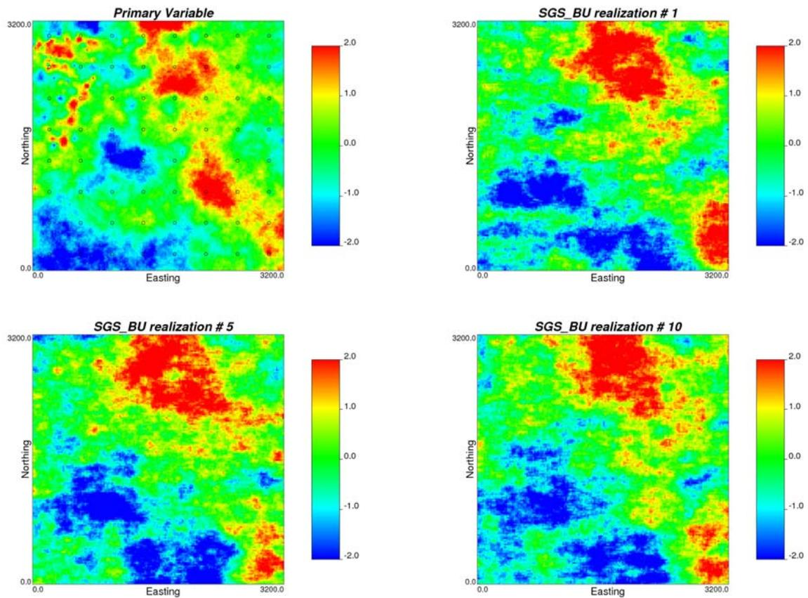
Figure 5: The primary variable (reference, up-left) and the SGS with Bayesian updating simulation realizations.
